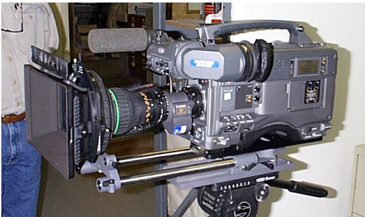
SONY DVW-700 with SAP-1, ARRI BP-6 Bridgeplate and ARRI MB-19 Matte Box
